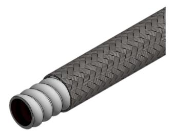
We recommend PTFE Easy Bend when you want a high durability and the application demands high chemical resistance and outmost flexibility. The hose is designed with a convoluted co-extruded inner tube from PTFE and an outer braid in stainless steel\*. In addition to our standard range we produce according to customer demands regarding dimensions, length and braid construction.
